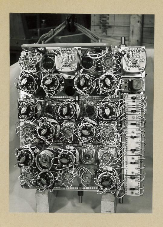
PAE IN TARGET-COMPONENTS CALCULATOR SERVO CHASSIS
