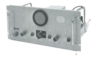
The receiver can be operated with a maximum of 12 crystal-controlled channels within a band of 7 Mc/s in the frequency range 156-174 Mc/s. The selection of 11 channels is effected by means of a switch on the front panel, whereas at a distance the choice between two channels can be carried out by means of the built-in relay.
