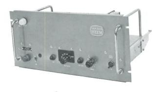
The transmitter can be operated with a maximum of 12 crystal-controlled channels within a band of 2.5 Mc/s in the frequency range 156-174 Mc/s.
