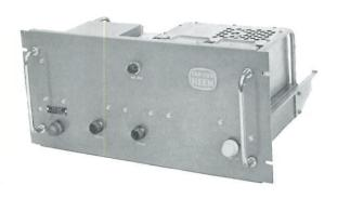
This power amplifier can be connected to the VHF-transmitter HTC 1205 without having to use separate switching lines. The HTC 1205 puts the power amplifier into operation when driving it with RF power.
