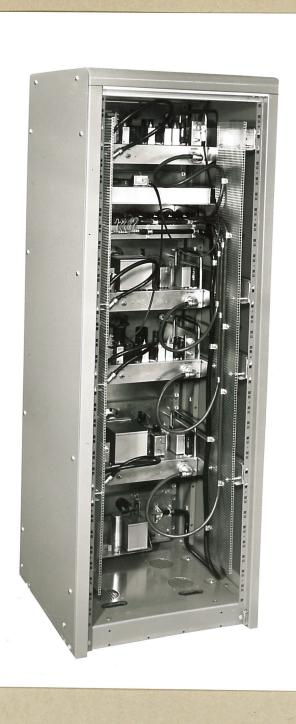
TYPICAL BASE STATION CABINET VHF TRANSMITTERS AND RECEIVERS (REAR VIEW)
