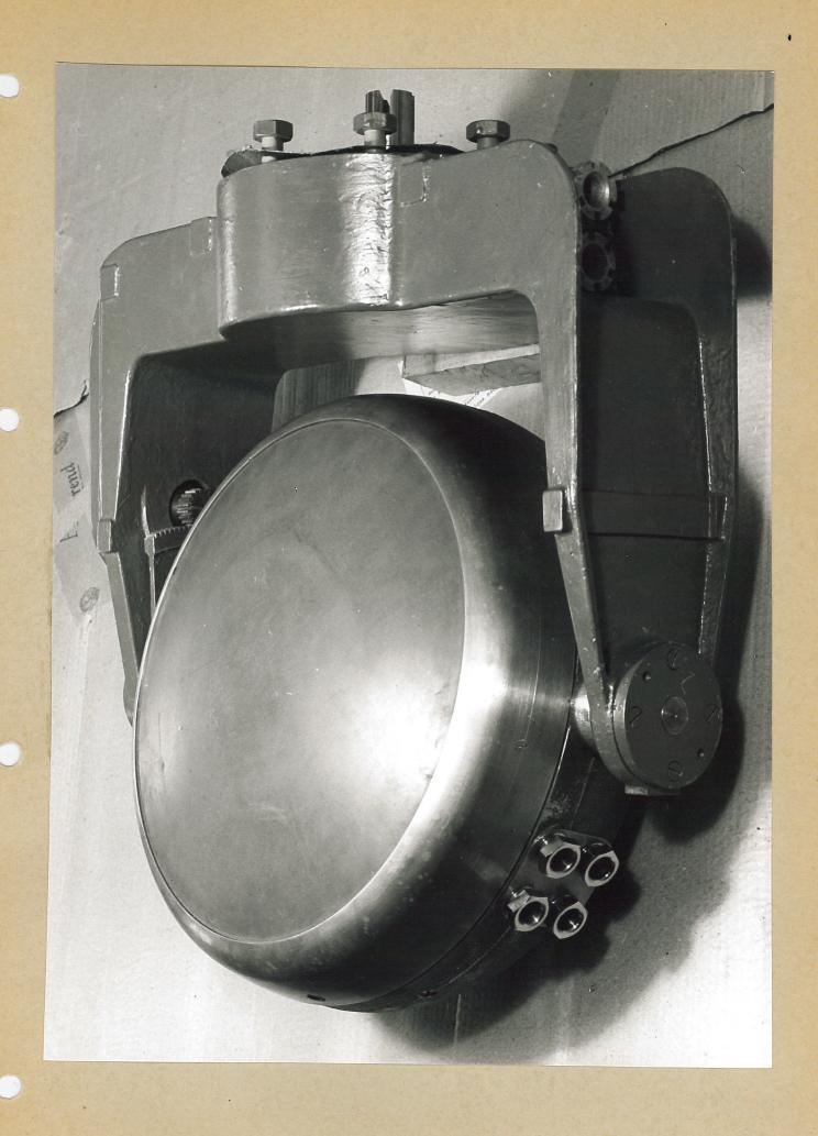
CRYSTAL TRANSDUCER IN BEHALF OF THE SONAR EQUIPMENT
